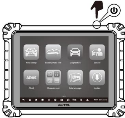
Figure 5-3 Power up the Tablet
